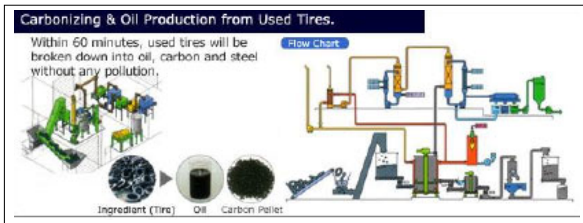
Figure 10: The pyrolysis process – schematic presentation of a system
